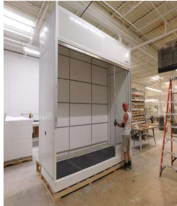
Install the (Sliding Door K) into the Door Frame .
