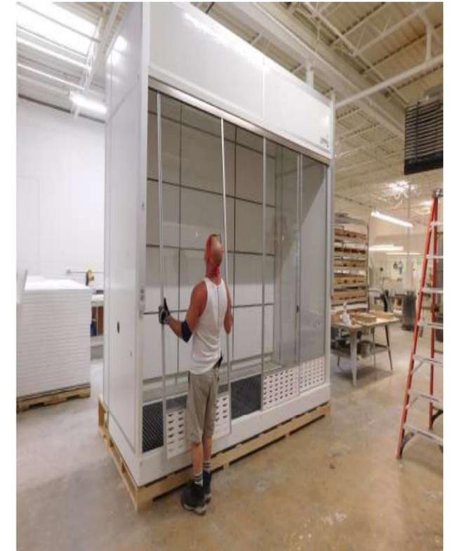
Install the (Sliding Door M) into the Door Frame .
