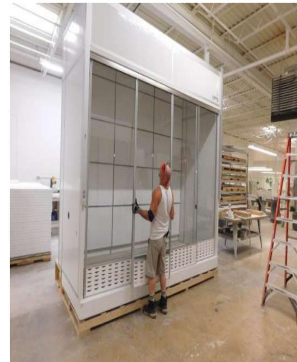
Install the (Sliding Door J) into the Door Frame .
